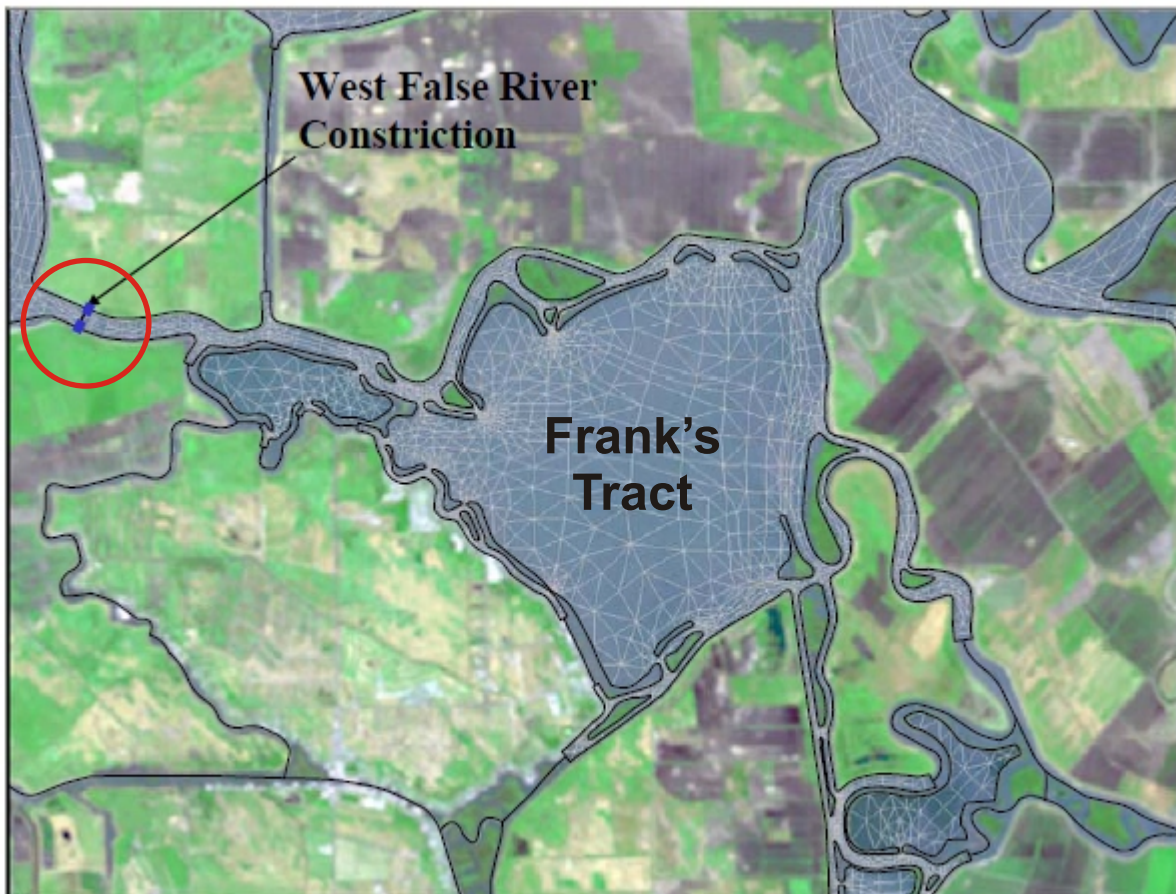
Figure 2-2 Grid for West False River Constriction Alternative 1.
