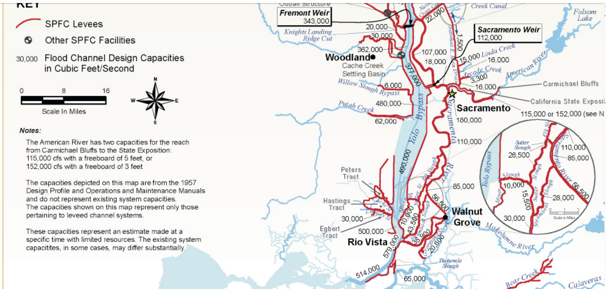
Figure 3-2. Design Flood Flow Capacities Within the Sacramento River, Bypasses, and Major Tributaries and Distributaries in the Sacramento River Basin
